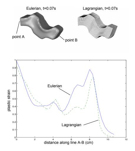
Figure 5. Effective plastic strain level at t=0.07s
