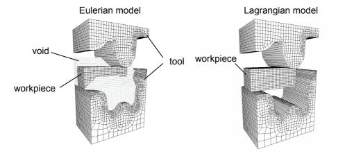
Figure 3. Eulerian and Lagrangian forging models
