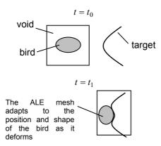
Figure 1. Moving ALE-mesh in impact simulation
